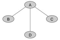
Figure 22.3a Low-redundancy network
